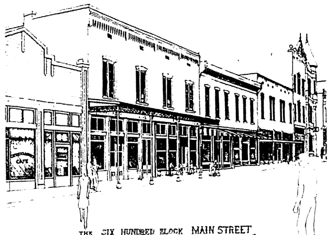
Figure 1. Inappropriate storefront alterations over the years—metal cladding, oversized signs and canopies—have detracted from the character of this historic district in Van Buren, Arkansas. A carefully considered rehabilitation plan for Main Street, including the removal of poorly designed signs, false fronts and the selection of an appropriate exterior paint color palette, serves to enhance the visual environment and preserves the district's sense of time and place. Photo above: Bob Dunn; Drawing, David Fitts
